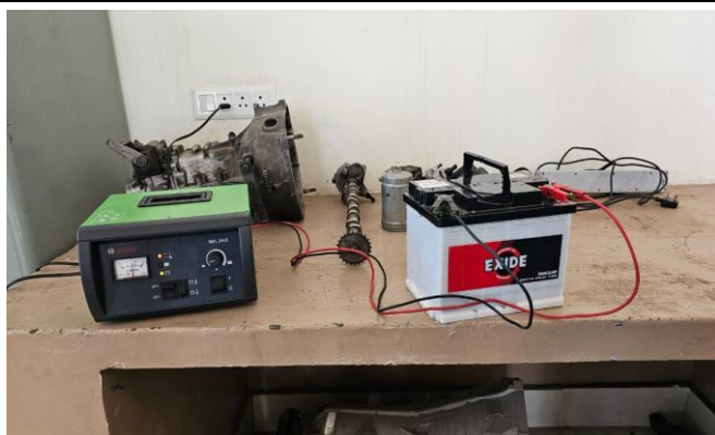
Fig. 8 Charging the Auxiliary battery using DC Charger
