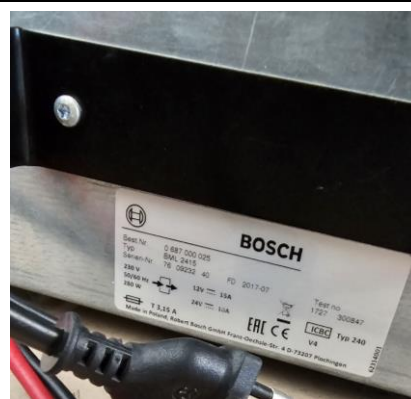
Fig. 9 Charger Specifications – BOSCH 12V DC Charger
