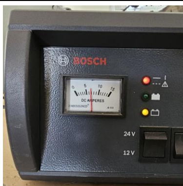
Fig. 10 Available charge after charging for 3 Hrs
